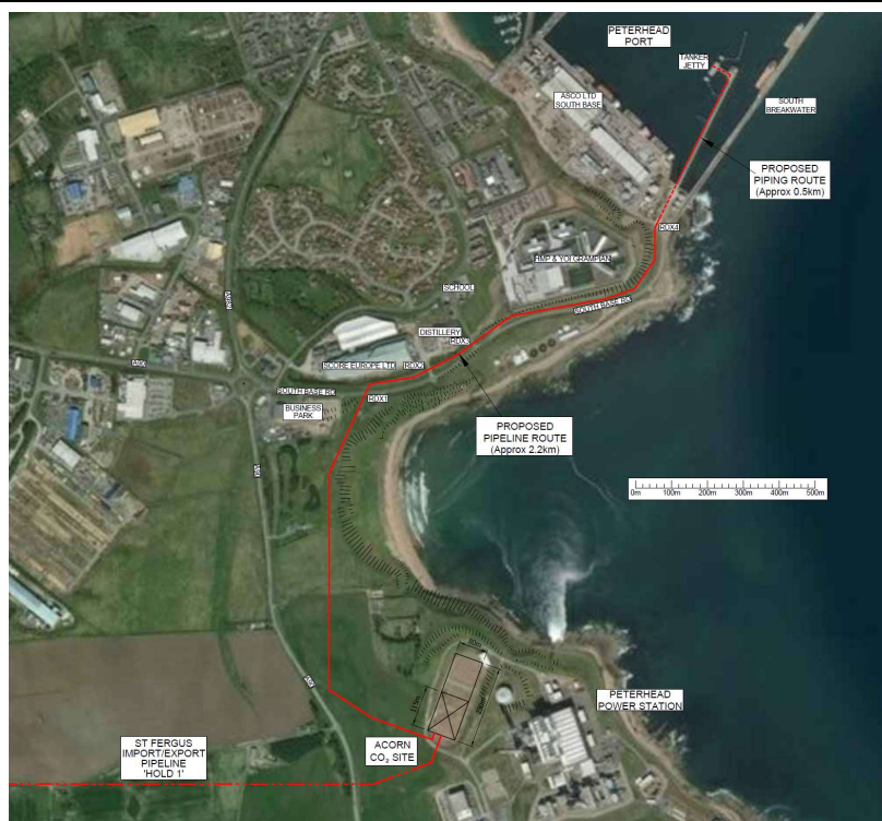
Figure 1 Illustrative pipeline route corridor for CCS development between Peterhead Port and Peterhead Power Station
