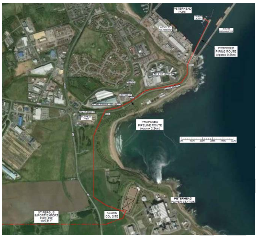
Figure 1 Illustrative pipeline route corridor for CCS development between Peterhead Port and Peterhead Power Station
